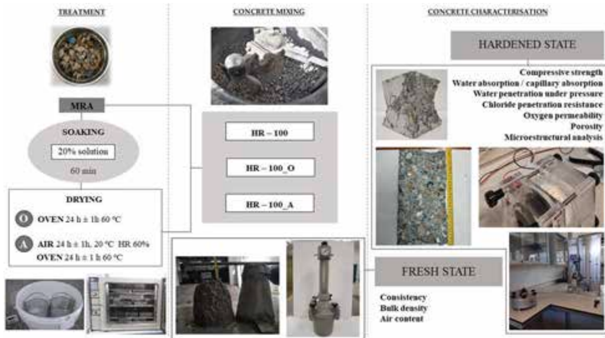
Fig. 1. Concrete manufacture, curing and characterisation.
