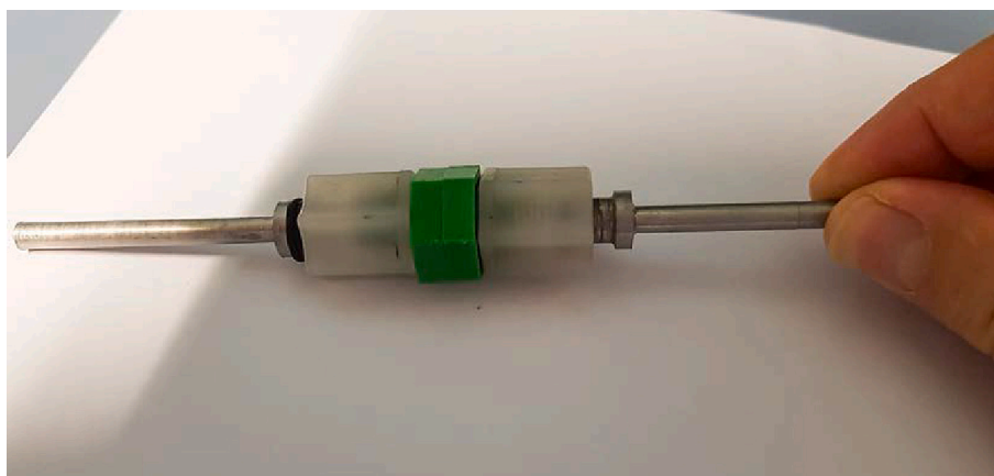
Fig. 12. Final result of the body inserted in the newly designed Swagelok® cell. An improvement in the design for the manufacture of supercapacitors is achieved by ensuring parallelism and the correct connection of the elements that make up the supercapacitor without jeopardising its structural integrity.
