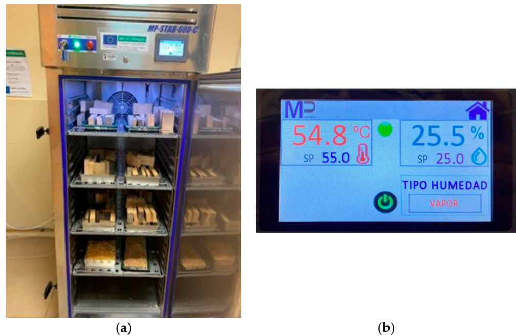
Figure 1. Climatic chamber device (a) and the screen for selecting the temperature and the relative humidity (b).
