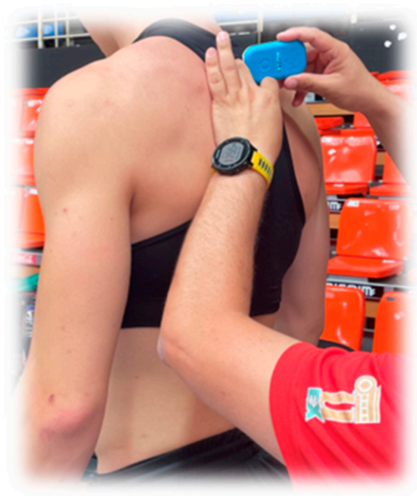
Figure 1. Positioning of the ID in the interscapular area by means of an anatomical harness.
