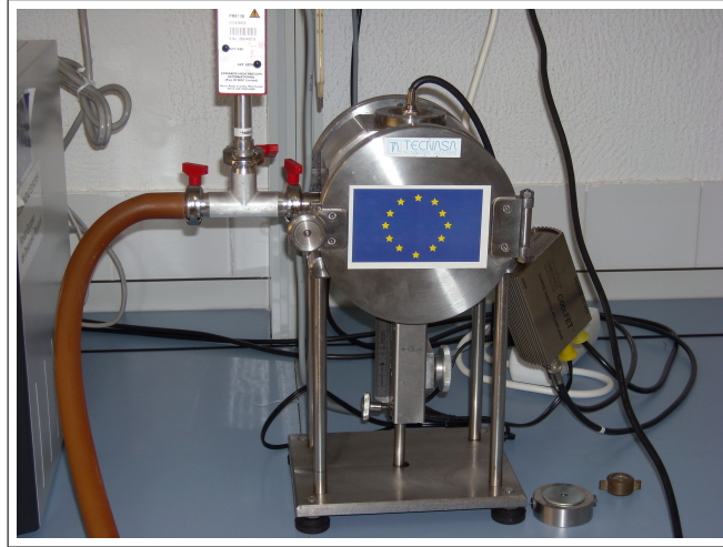
Figure 3.1: Semiconductor chamber designed and characterized at the University of Extremadura.
