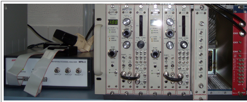
Figure 4.13: Comparison of the electronic modules used by the analogical coincidence system (left side) with the digital module (right side).
