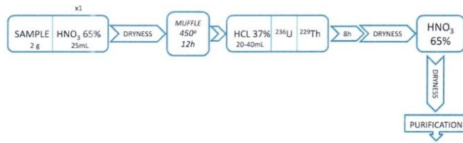
Fig. 1. Acid leaching procedure for carbon samples.
