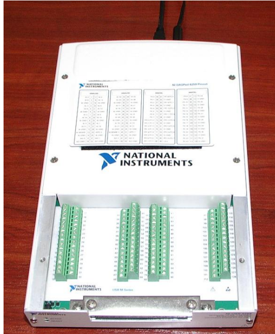
FIGURE A.5: Picture of NI 6259 Data Acquisition Board
