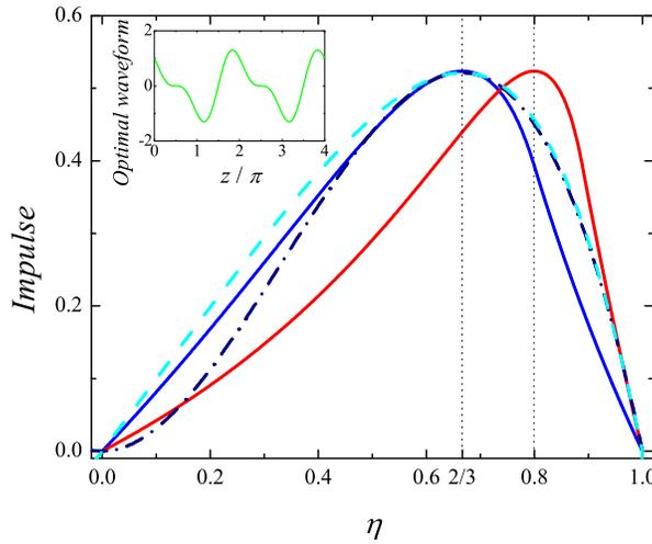
FIG. 4: (Color online). Impulse functions  $I[f_{\varphi_{eff}=0}^*](\eta)$  [blue (black) line, Eq. (9)],  $I[g_{\varphi_{eff}=0}^*](\eta)$  [red (gray) line, Eq. (12)],  $3.37(I[f_{\varphi_{eff}=\pi/2}^*] - 1)$  [dashed line, cf. Eq. (6)], and  $3.52\eta^2(1 - \eta)$  (dashed-dotted line) versus  $\eta$ . The inset show the optimal waveform  $\cos(z) - 0.5 \sin(2z)$ ,  $z = \{t, x\}$ , for both temporal and spatial biharmonic forces [Eqs. (1) and (2)].
