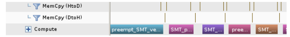
Fig. 1. A profiler capture showing the eviction (and re-launching) of five kernels. Three transfers are required to evict a running kernel and launch a new one.
