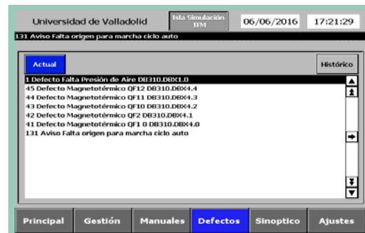
Figura 16: Defectos Panel Operador
